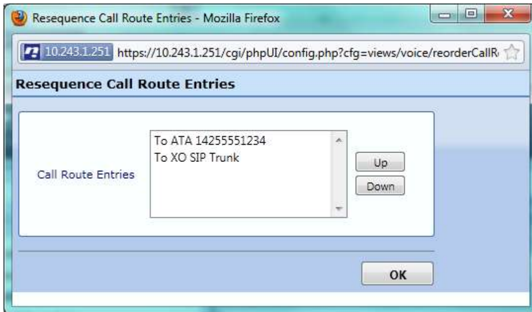
Figure 45 Route Table Ordering for calls to ATA
