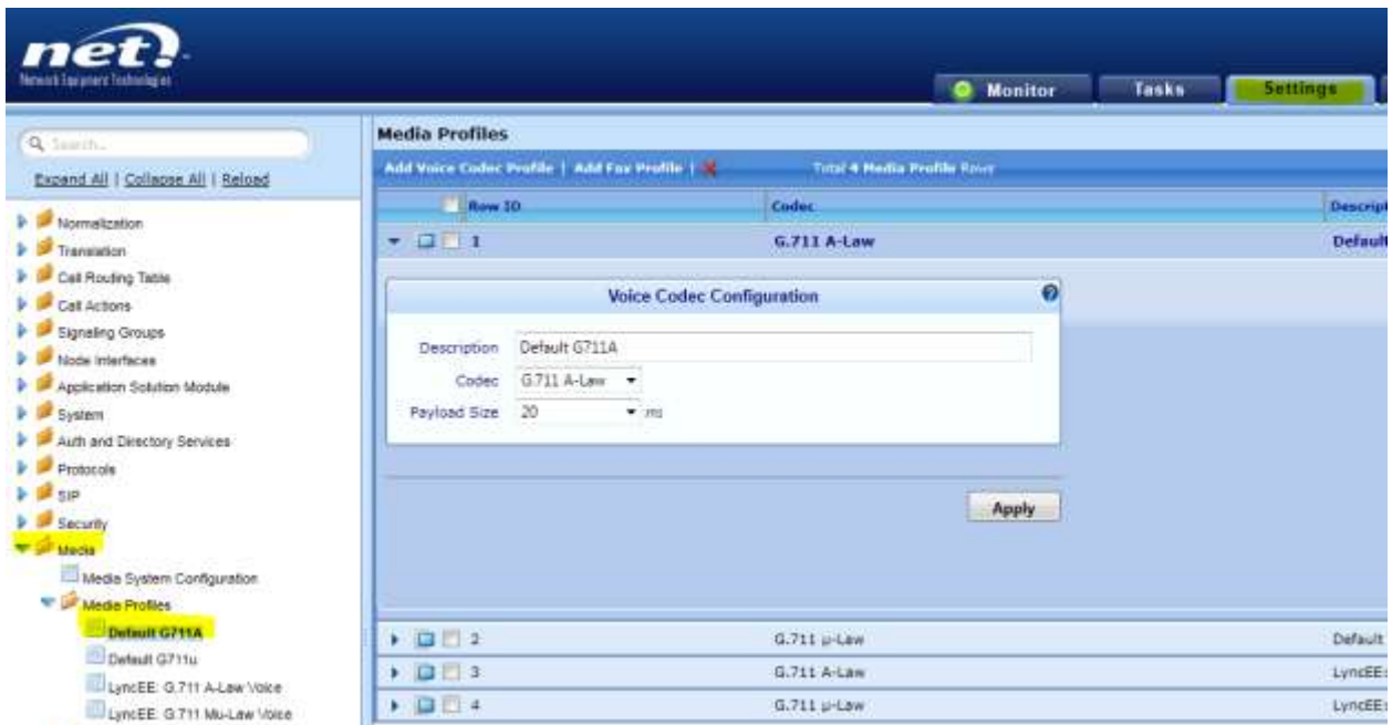
Figure 27 Typical G711Alaw Codec Settings
